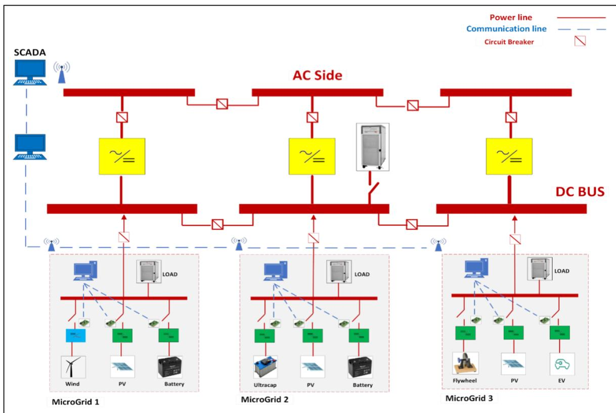
Figure 2: Microgrid structures and the suggested energy management model
