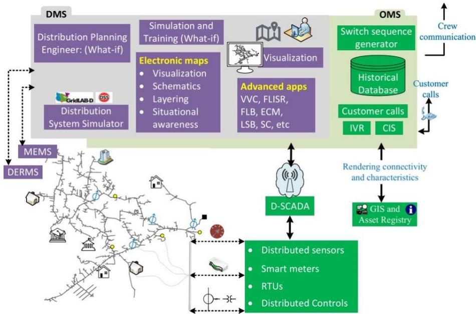
Figure 1: Advanced Distribution Management System ADMS [8]
